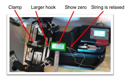
**3.3b Pulling the string:** Connect the smaller hook of the calibrator into the gripper and start to pull string. After reach to the setting value, calibrator and motor display show their tension data. See as follows:
